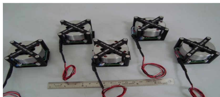
Sona SPEED Research and Development centre in Department of EEE Delivered 5 Nos. of Miniature reaction wheel (MRW) to M/s Indus Teqsite for use in future Student satellite missions.
